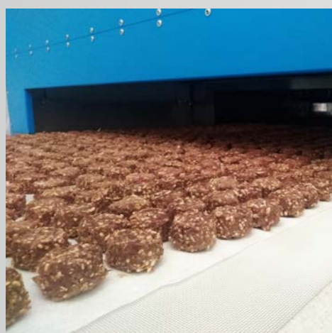
▶ RF equipment for pet food 600 kg/h throughput
