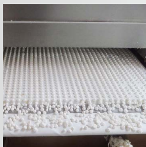
▶ RF equipment for meringues 500 kg/h throughput
