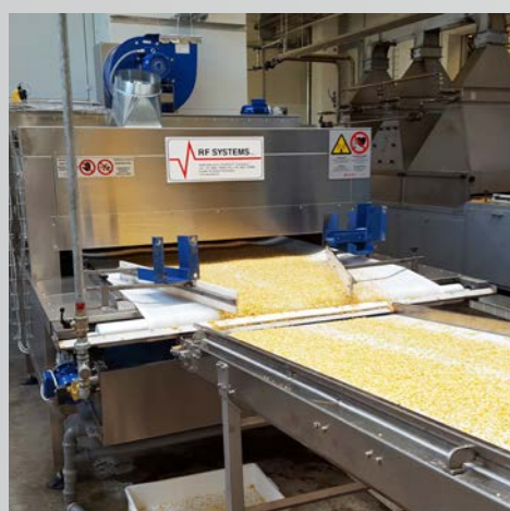
➤ Sanitization of corn 1000 Kg/h throughput
