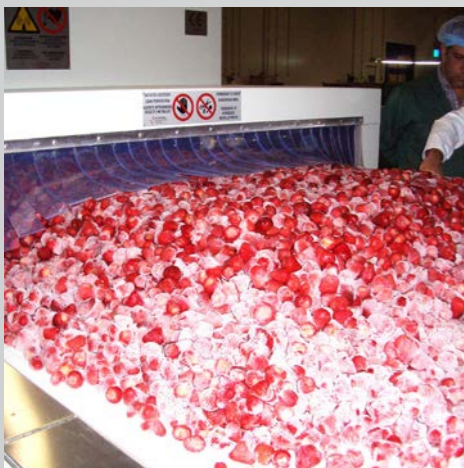
> Defrosting of IQF strawberries 1000 Kg/h throughput
