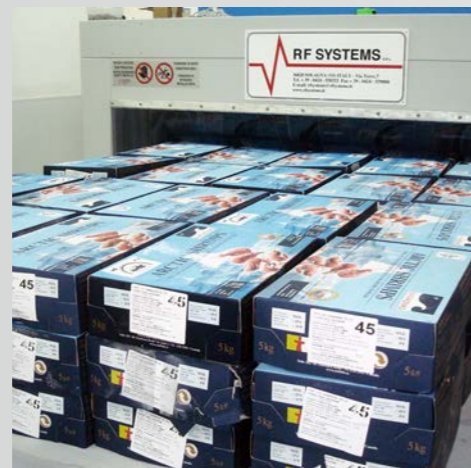
> Defrosting of packaged shrimps 1500 Kg/h throughput
