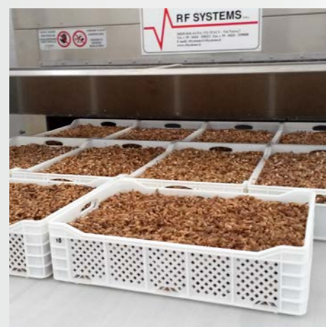
▶ RF drying of shrimps' shells 600 kg/h throughput
