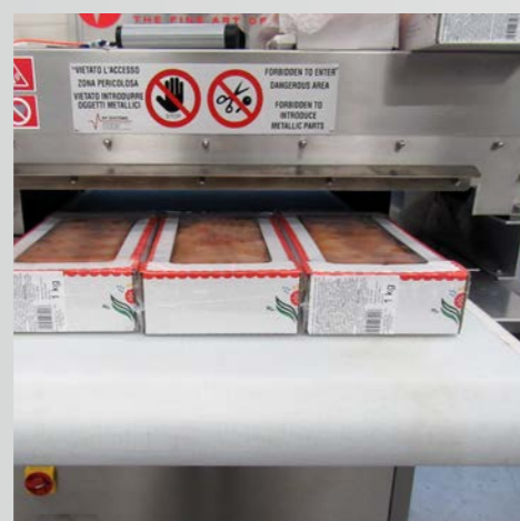
➤ Pasteurization of packaged croissants 300 Kg/h throughput
